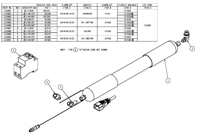
Figure 53 Heated Piston to DV Hose Assemblies
